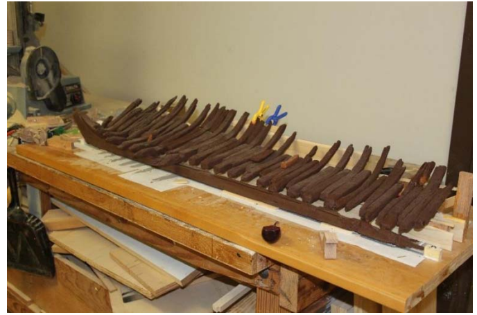
3-D model of the 220 S. Union Street Ship printed from digital scans. Courtesy of Conservation Research Laboratory, Texas A&M University
