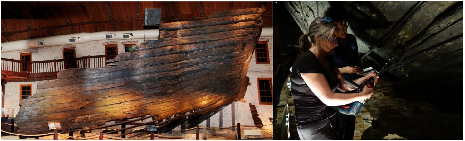
Left, ship's hull on display at the Western Australian Shipwrecks Museum in Fremantle (P.E. Baker, Western Australian Museum); right, Marta Domínguez-Delmás and Aoife Daly extracting a sample from the hull with a dry-wood borer driven by a power-drill. (Wendy van Duivenvoorde, Flinders University).
