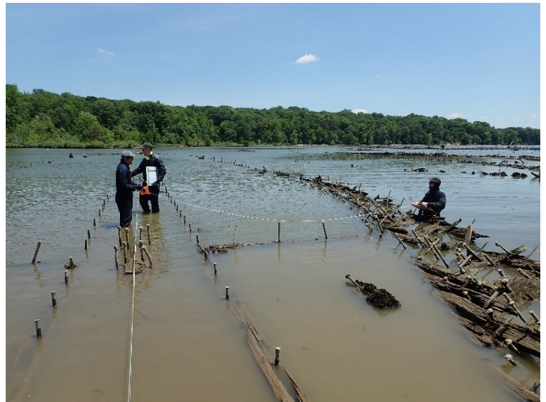
Students diligently work using the baseline-offset method to map Bayou Teche. (Jill Schuler and Lindsay Wentzel/ECU Program in Maritime Studies).
