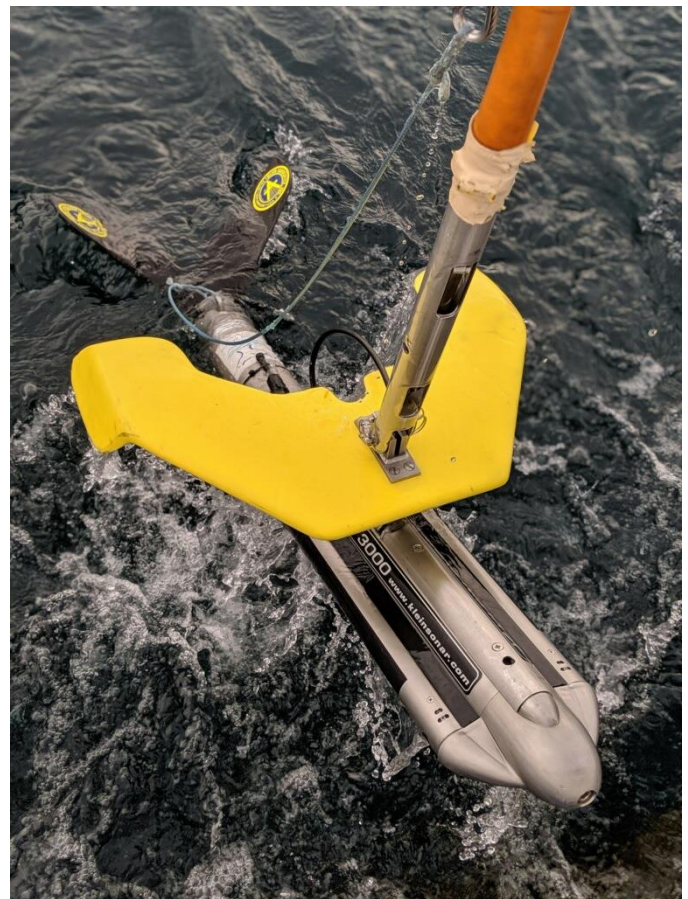
Remote sensing data was collected with NOAA's side scan sonar system and onboard multibeam ecosounder. Here, NOAA's Klein 3000 is launched from R/V Storm, 9 Sept 2019. (U.S. Navy photo by Alexis Catsambis/Released).
