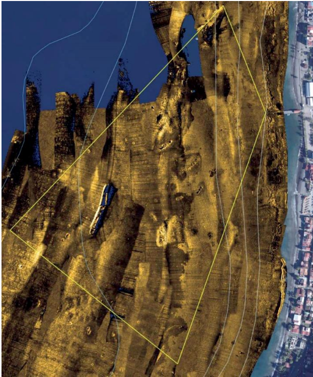
Side-scan sonar survey in Saint-Pierre Bay. Imaging by F. Leroy, DRASSM (French Department of Underwater and Submarine Archaeological Research).
