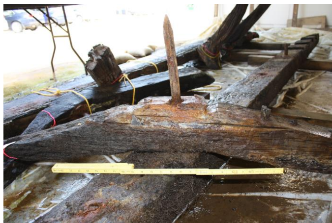
Floor attached to keelson (keelson is upside down). Photo courtesy of SEARCH, Inc.
