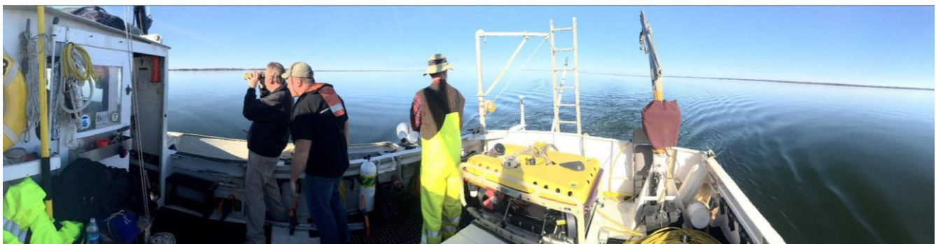
SUPSALV and IMH observing autonomous underwater vehicle as it conducts side scan sonar to map wreck and debris field (U.S. Navy photo by George Schwarz/Released).
