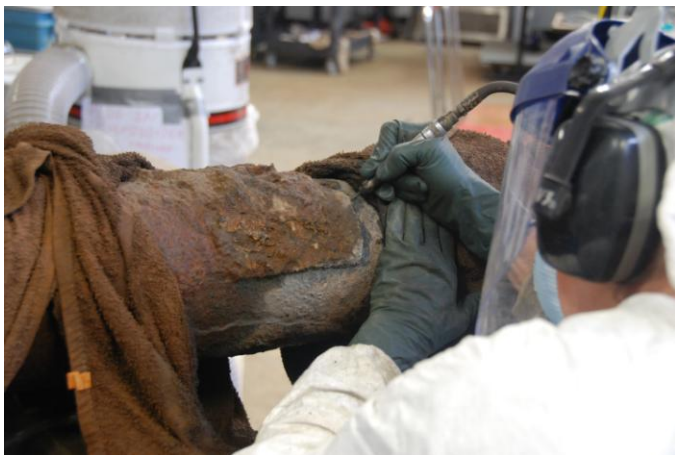
Conservator cleaning cannon surface using an air scribe.
