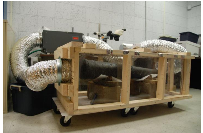
Lexan (polycarbonate) drying enclosure for a 1-pounder cannon.
