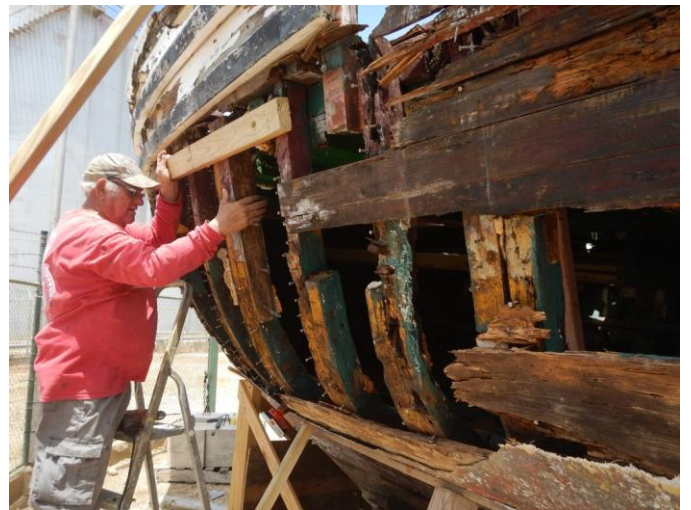
One of the shipwrights, Johnny Craane, inspects the frames for deterioration. Photo by P. Holian.
