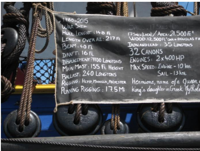
Statistics and other information about Hermione as presented dockside. Photo by the author.
