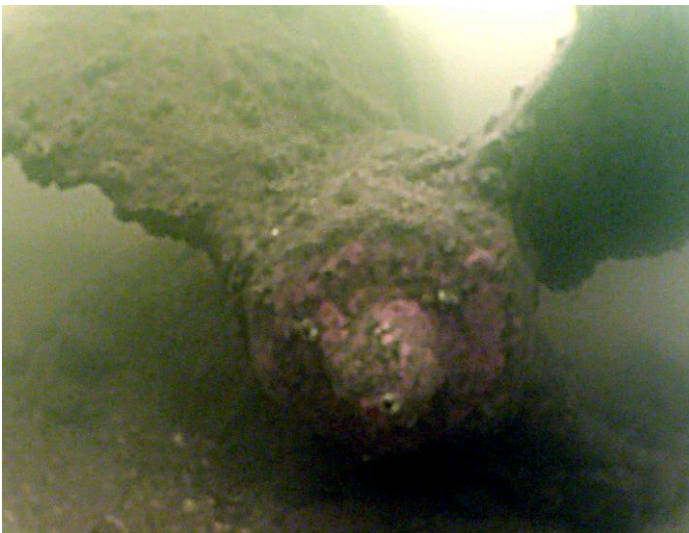
City of Tampa: The running gear terminates with the intact four-bladed propeller. Photo by the author.
