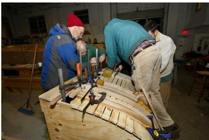
Volunteers clamping steam-bent frames to a mold. The frames cool into the proper position. The frames were then installed after the planking was finished. Photo by ASF.
