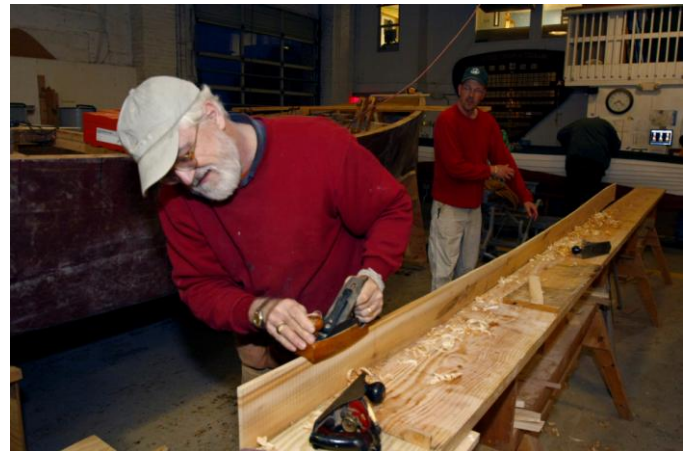
The boat was built using a shell-first technique, in which the hull planks are applied first followed by the frames. Here volunteers are planing hull planks on the planking bench. Photo by ASF.
