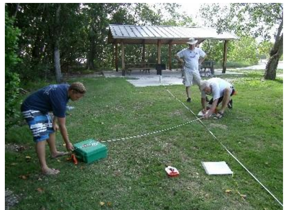
E. Reger and J. Gorman practice trilateration with J. Smailes supervising. Photo by the author.
