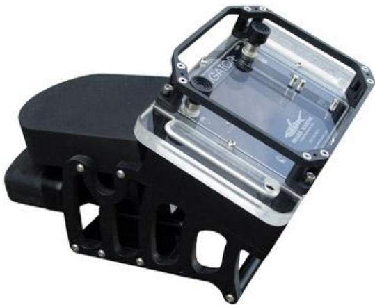
The Shark Marine Navigator unit features multi-frequency sonar with profiling and sector mode, surface navigation with GPS, optional digital HD camera, multi-beam sonar, magnetometer, and sub-bottom profiler. Image from www.sharkmarine.com .
