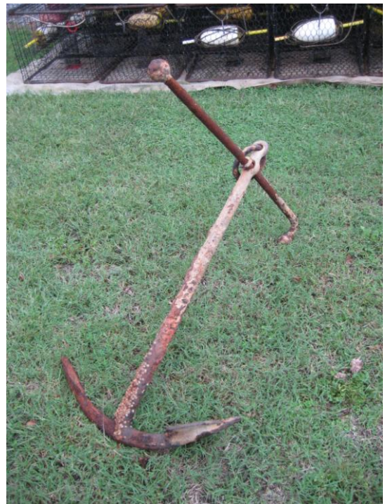
19 th -century iron folding stock anchor recovered by landowner, B.T. Smith, near White House Landing. Photo by J. Smailes.
