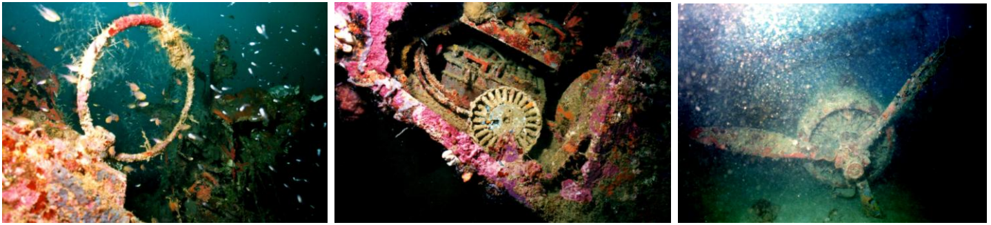
Diagnostic features of the Mavis: left, ADF ring; middle, machine gun ammunition ring; right, engine and propeller.
