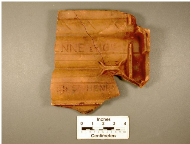
Marseille roofing tile. Photo by the author.
