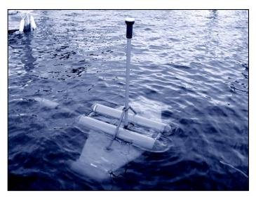
Marine Magentics SeaQuest 3-Axis gradiometer during initial testing in the Patuxent River. Photo by T. Nowak
