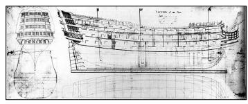
The lines of HMS Victory, a 100-gun first-rate ship of the line. www.shipmodeling.ru/imgup/img\_gry1o1193431809.jpg
