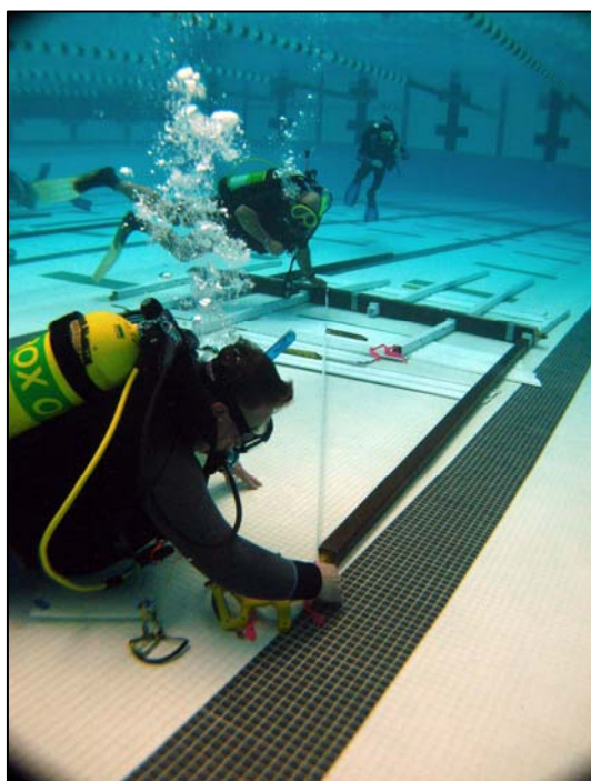
Divers from the Massanutten Chapter of ASV practice trilateration mapping underwater. Photo by the authors.
