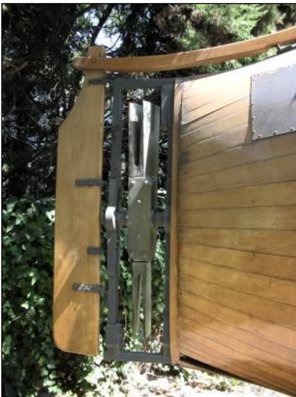
Above: The Ictineo, Spain's first submarine, 1859. Built of olive wood she was designed for coral fishing and oceanographic research. Below: The propeller and rudder on the Ictineo.
