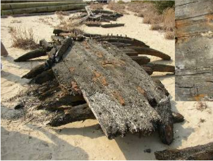
Fort Story Wreck,, Virginia Beach, Virginia. Inset shows detail of caulking. Photo by the author.
