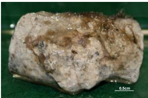
Unidentified specimen recovered from the deck of CSS Alabama and thought to be putty, machine grease, or "white lead." Lead (Pb) concentrations through the thickness of the specimen shown on the right. No lead was detected at the surface, but concentrations increased towards the center of the specimen (#3). Moreover, the brown surface film contained four times the maximum Pb value in the specimen itself. Image by Thermo-Fisher, Co.
