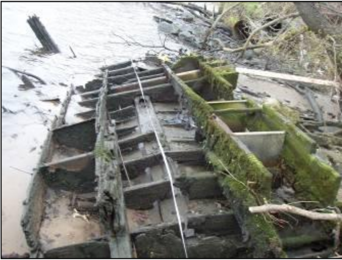
Salisbury LCVP, view aft with engine mounts right and left of centerline. Photo by T.Berkey.
