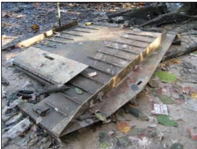
Salisbury LCVP, open ramp at bow end with view port down. Photo by J.Gardner.
