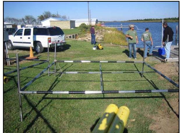
One of the 10-foot by 10-foot stainless-steel grids used to control the excavations at the wreck site (photo by M. Krivor)
