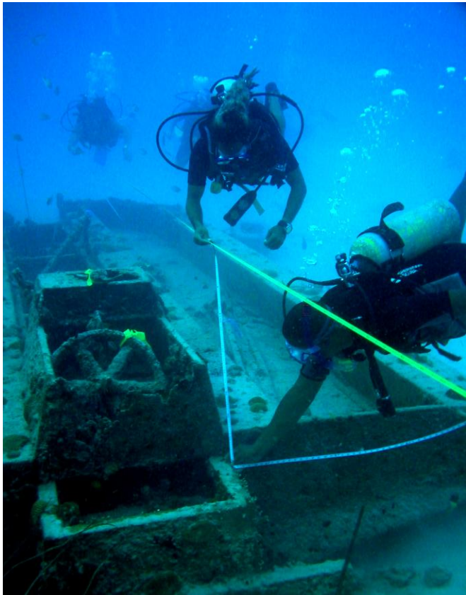
Trilateration: pulling the tape tight while staying clear of the baseline is harder than it looked on dry land. Photo by Dennis Knepper.
