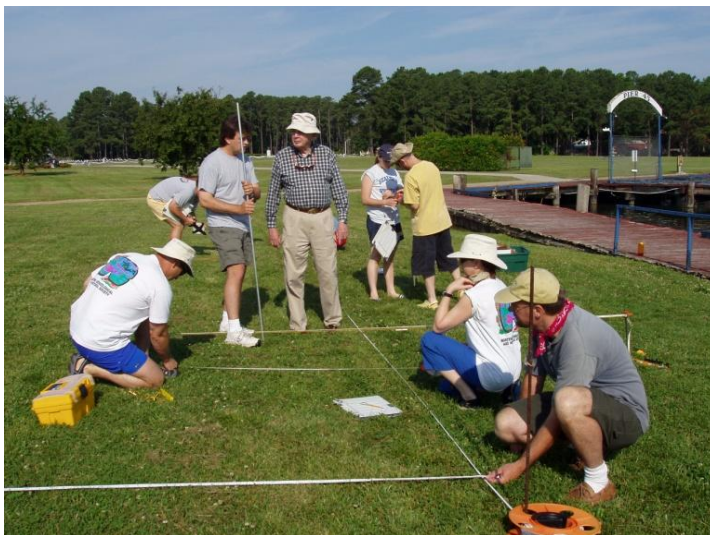
Kurt Knoerl and Tom Berkey demonstrate the trilateration survey method on dry land. Photo by Michele Anthony.
