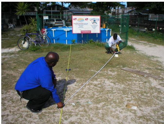
Field school participants practicing trilateration on dry land: this looks easy! Photo by Dennis Knepper.
